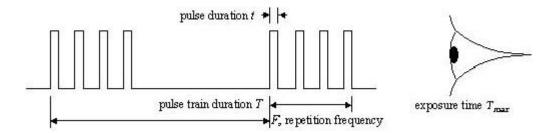
There are three rules that limit the MPE per pulse for a train of laser pulses:
